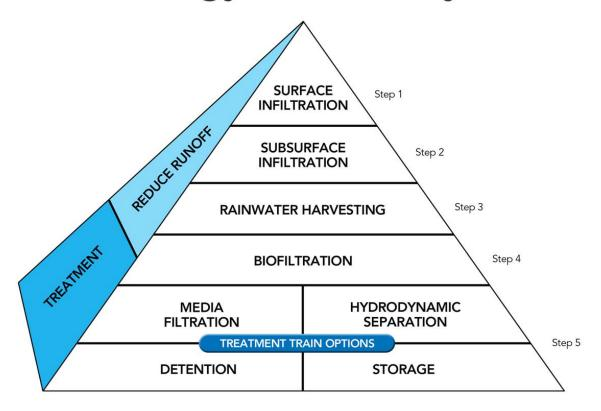
The stormwater community is witnessing the burgeoning implementation of green infrastructure and Low Impact Development (LID) practices. A systematic approach is necessary to identify an LID-based technology suitable for a given site. The LID technology selection pyramid illustrates a step-by-step approach to identify technologies to meet the fundamental goals of LID – runoff reduction and water quality treatment.
