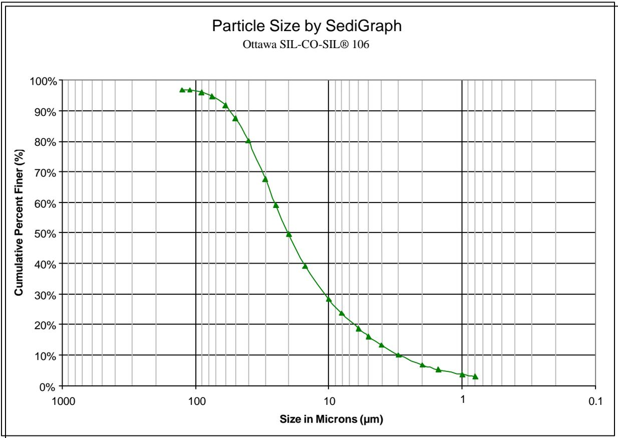
**Figure 1: Sil-Co-Sil 106 Particle Size Distribution (source U.S. Silica)**
